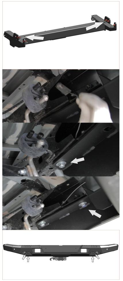
11. Install bumper bracket on the car frame. Fasten with bolts M12x24x1,25 with washers M12x24. Do not tighten threaded connections.
