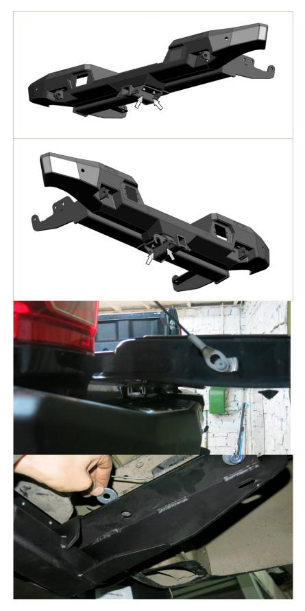
12. Instal the towing bar bracket on the car and screw with 2 bolts M12x1,25x30 and washers M12x24 on several turns.
