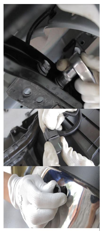
1. Unscrew tension bolts of the standard bumper the left and right of the vehicle frame. Dismantle the bumper
