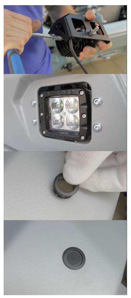
5. Install the lights (18) onto the brackets (4). Align the position of the lights and tighten screw joints
