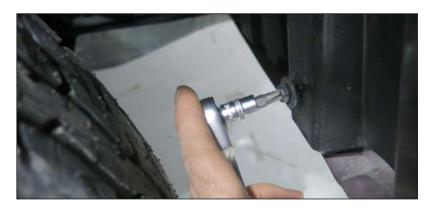
9. Unscrew the screw which attaches mudguard to bracket (see step 7 No. 2).
