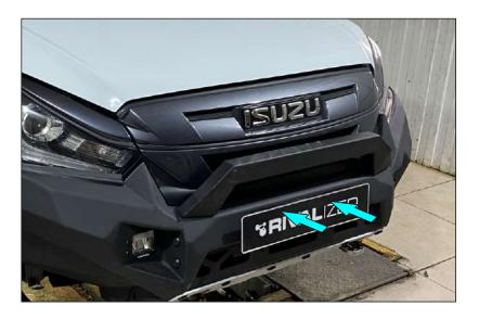
30. Install license plate bracket (pos. 3). To do it, apply it to the bumper first, then mark locations for drilling and then drill mounting holes.
