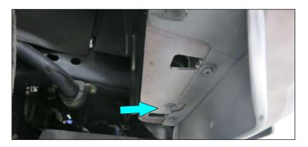
10. Unscrew the nut which attaches mudguard to bumper (see step 7 No. 3).
