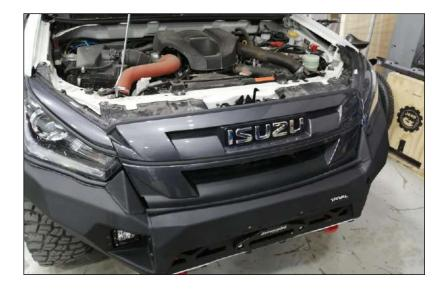
31. Install radiator grille using the factory hardware (see step 3).
