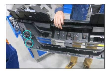
5. Remove radiator grille by detaching 2 latches from bumper on each side
