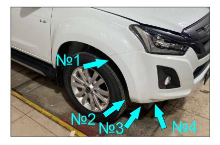
7. Unscrew all fastening elements on **each** bumper sides (see step 8 – step 11).
