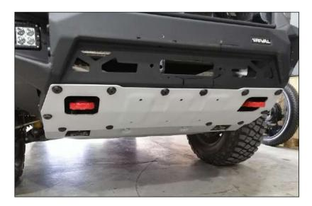
27. Install underguard plate (pos. 8) to aluminum bumper body (pos. 1) fix it with M10x30 screws (pos. E) and countersunk washers (pos. N).
