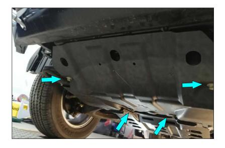
19. Unscrew 4 bolts and remove engine skid plate.
