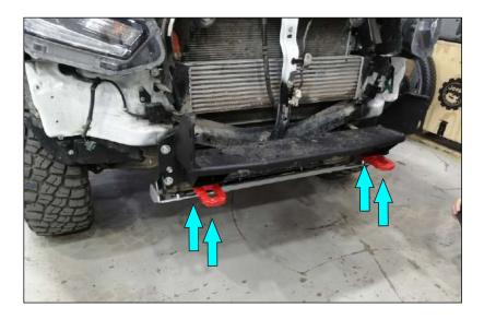
21. Mount recovery points (pos. 9) to winch bracket (pos. 2) by using M10x40 bolts (pos. B) and penny washers 10 (pos. L).
