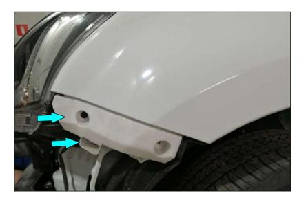
15. Remove plastic brackets which fasten the factory bumper on each side.
