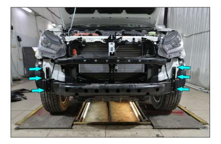
16. Remove brackets which fasten mudguards by unscrewing 3 bolts on each side.
