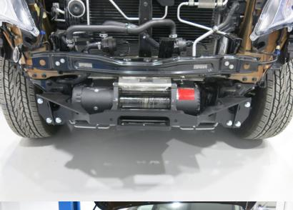
30. Install the winch bracket onto the vehicle. See paragraph 25.
