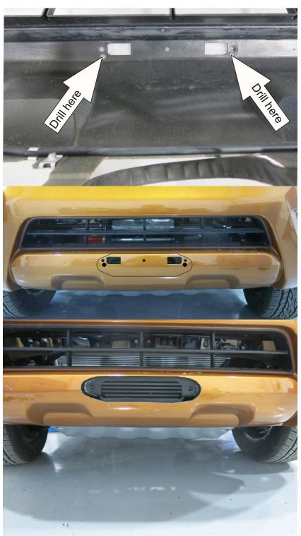
26. Temporarily install standard bumper for pad eye hole spacing. Mark the hole for pad eye fasteners on the inside of the bumper along the winch bracket. 27. Remove the bumper.
