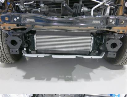
24. Install adapters (pos. 4 and 5) onto the vehicle frame using standard fasteners from the frame booster. Do not tighten screw joints.
