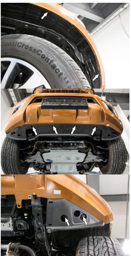
8. Unscrew 2 self-tapping screws of the bumper clamp in arches on the left and right.
