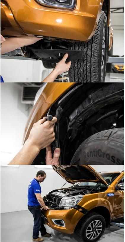
11. On the bumper inside unscrew 2 retaining nuts of the bumper skirt side and dismantle the bumper skirt side.
