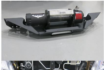
29. Remove the winch bracket from the vehicle, install the winch and pad eye onto the bracket and secure with bolts from the set of winch and pad eye.
