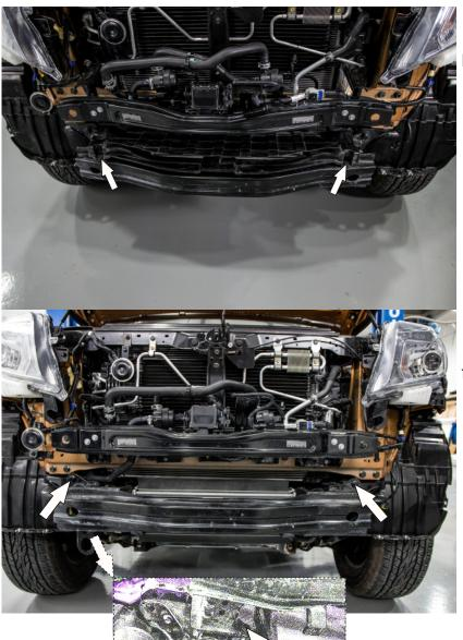
18. Remove the air intake clips. Dismantle the air intake.
