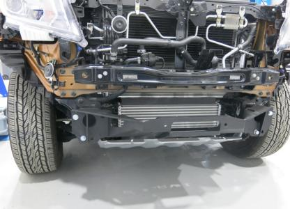
25. Install the winch bracket (pos. 1) onto the vehicle. Secure to adapters and frame boosters using bolts M12x30 (pos. 9), nuts M12 (pos. 11) and washers (pos. 12). Adjust the winch bracket. Tighten all screw joints, including adapters and frame boosters.
