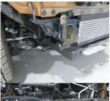
23. Install right frame booster (pos. 3) onto the vehicle frame, secure with standard bolts with installation of standard towing eye. Do not tighten screw joints.
