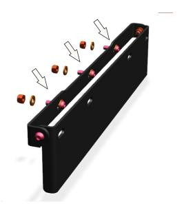
33. Install license plate (pos. 1) onto the bumper using 3 screws M6x20, nuts M6 and washer 6.
