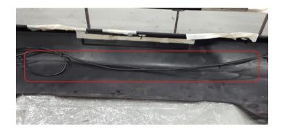
28. Fix wires inside the bumper, as red zone shown, using pressure sensitive liner (pos. 24).
