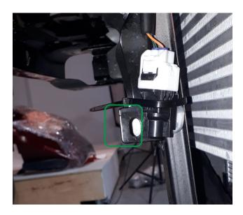
18. Check if winch stuck on the center part of the bracket..
