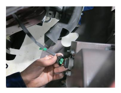
9. Carefully dismantle the bumper. Pull the bumper edge by unlatching the latches, moving from the bumper edge to the center.
