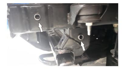
13. 11. Place bushings (pos. 7,8) into the chassis, on the left and right side of the vehicle, as shown.
