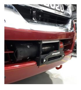
30. Try the bumper on the vehicle, and check that winch doesn't pull out and contact the bumper.
