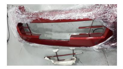
29. Make sure, that wires do not handicap to cut the bumper. Carefully cut out marked area, using angle grinder.
