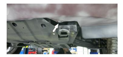
35. Install the bumper onto the vehicle and fix it, using bolts M8, adjusting washers M8 and nuts M8.
