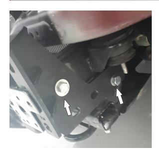
14. Install the bracket (pos.3) on the left side of the frame, as show, using bolts M10x100, bolt M12x110, adjusting washer M10 and washer M12.
