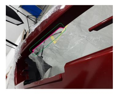
31. In case if bumper doesn't fit, depends on winch, cut out inner top part of bumper, as shown.
