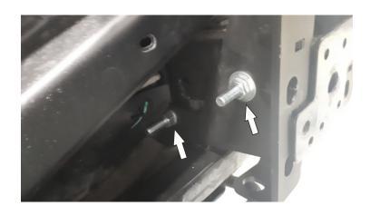
15. Install the bracket (pos.5) on the left inner side of the frame, as show, and fix it using adjusting washers M10, adjusting washer M12, nut M10 and nut M12.
