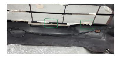
27. Carefully cut tie wraps, inside the bumper, that fixed wires with bumper fittings, as green zone shown.
