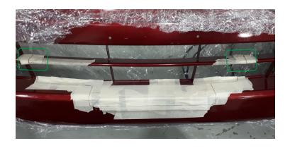
26. Measure width of radiator grille area to cut out, following winch dimensions, Stick masking tape on the grille, and mark cut line, as shown.
