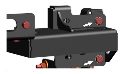
17. Install winch bracket (pos. 2) and winch on the brackets, using 2 bolts M12x40, washers M12 and nuts M12 on the both sides.
