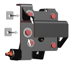
20. Fix left side of th winch bracket, using bolts M12x40, insert nuts M12(pos.9), adjusting washers M12, as shown.
