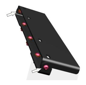
34. Adjust license plate angle. Tighten all the joints.
