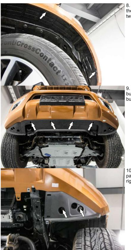
8. Screw out self-attack screws fastening the bumper in arches on left and right, two on each side.
