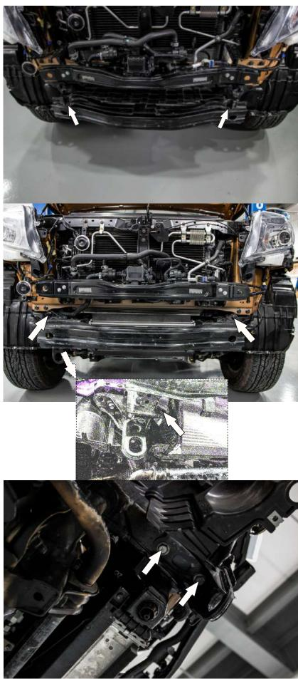
18. Remove clips which fasten the air intake. Dismount the air intake.
