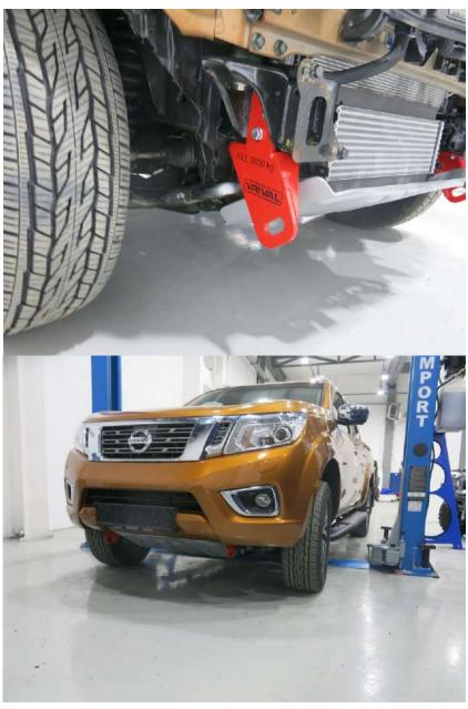
25. Fasten the towing loop (item 2) in lower part with standard bolts which fasten the towing eye.
