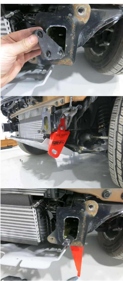
21. Insert captive pins 3xM12 (item.3) into the car frame on left and right.
