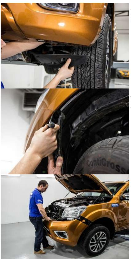
11. From the bumper inside, screw out 2 nuts which fasten the bumper skirt lateral part, and dismount the bumper skirt lateral part.
