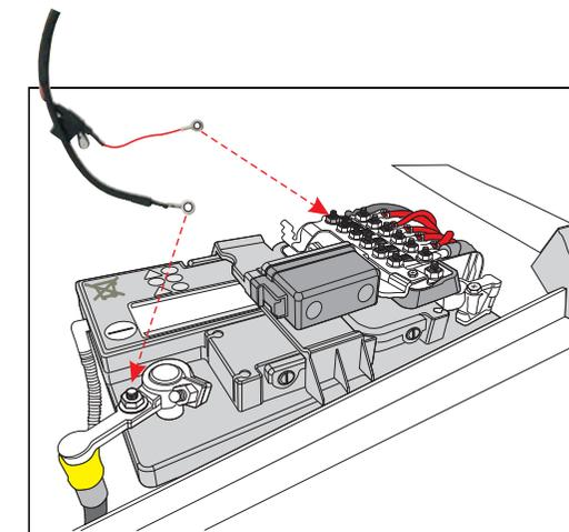
Diagram 6 - CONNECT VEHICLE HARNESS TO TERMINAL
