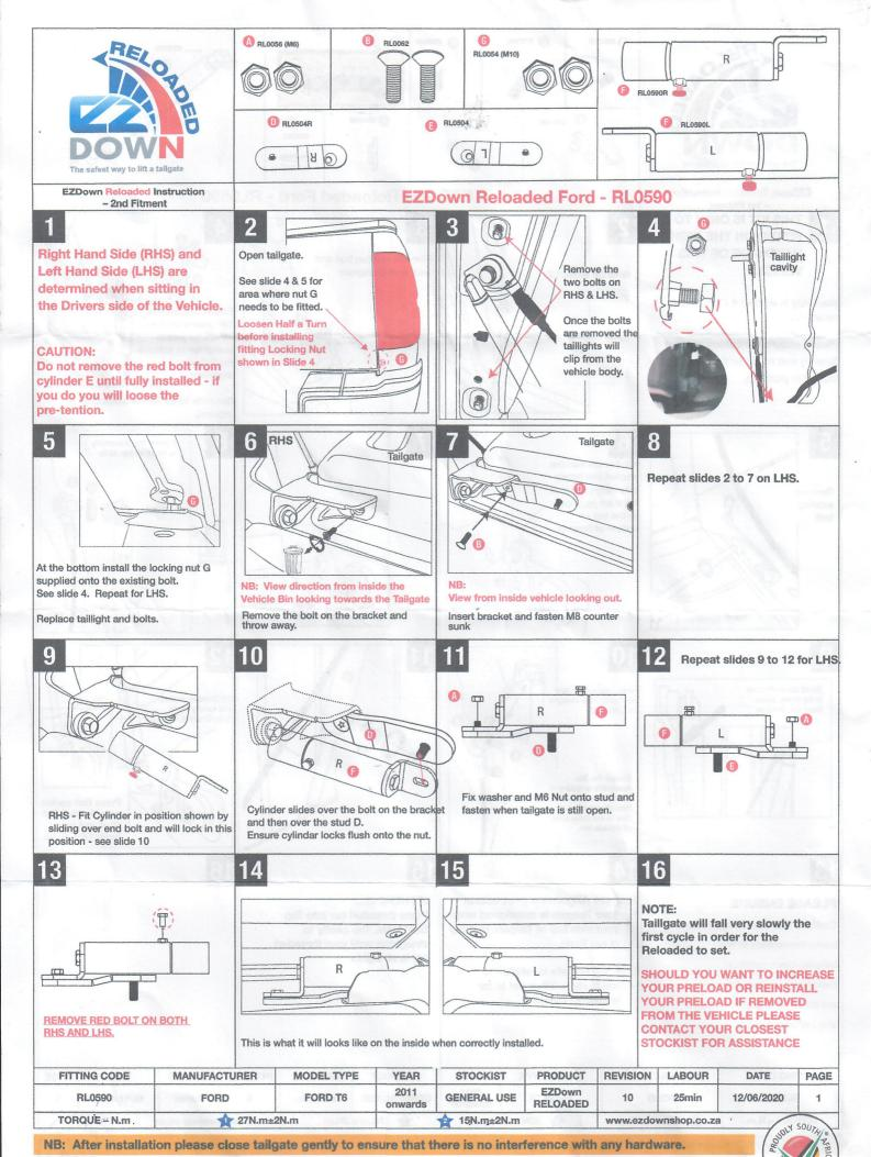
NB: After installation please close tailgate gently to ensure that there is no interference with any hardware.
